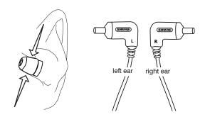
Make sure that the sleeve completely covers the earphone nozzle. If any part of the nozzle is exposed, the sleeve is not properly installed.
